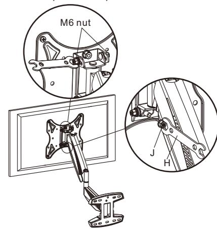
Make sure the plate is downward when tighten the nut
