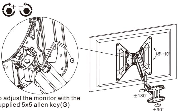
To adjust the monitor with the supplied 5x5 allen key(G)
