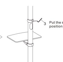
Put the stop block at proper position, fix it with allen key (3).
